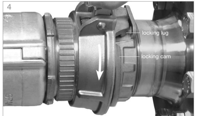
Lead female coupling with its locking lug to the locking cam of the male coupling. Do not use tools, hand force is sufficient.
