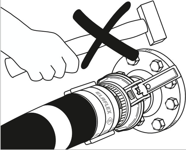
**Do not put the system into operation with an open lever.** If the lever is not fully closed, the coupling lock may not work. - Danger of accidental detachment, e.g. due to vibrations.
