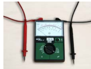
Ohmmeter: used for measuring 'M' hoses
