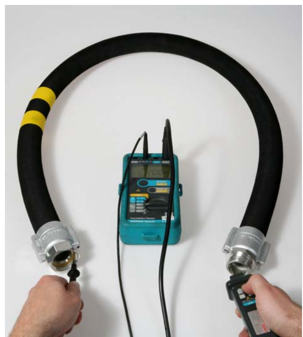
Electrical continuity testing
