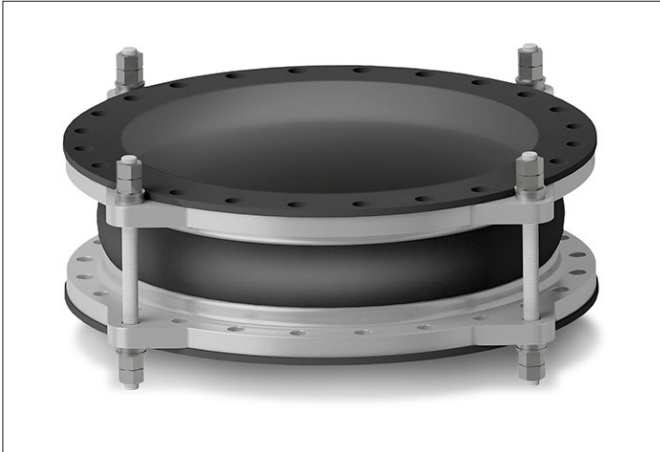
Tie rods with outer limitation type ZS in spherical discs and conical seats. – elongation limitation, lateral movement possible –
