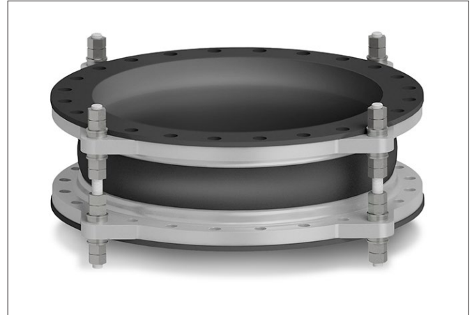
Tie rods with inner and outer limitation type ZSS inside and outside in spherical discs and conical seats. – elongation & compression limitation, lateral movement possible –
