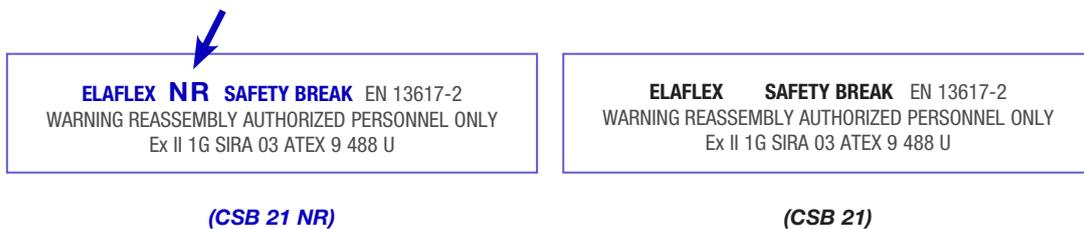
After separation **CSB 21 NR** cannot be reused. Even if reassembled, the coupling stays closed. The coupling must be replaced with a new one.
