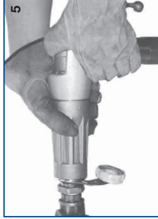
5 Unscrew GG10, note small release of gas.
