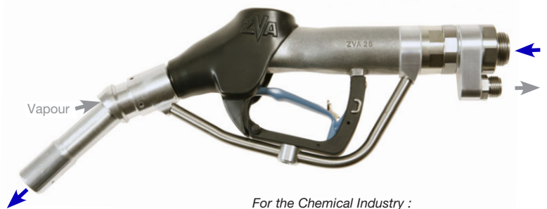
For the Chemical Industry : automatic nozzle ZVA 25 GR. Active, open vapour recovery for solvents. Refuelling rate max. 140 l/min.
