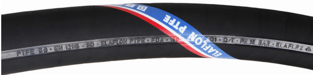
Example ELAFLO PTFE - max. 10^6 Ohm resistance between hose end fittings - max. 10^9 Ohm through the hose wall. According EN 12115 so far classified as \Omega hose, according EN 12115 : 2011 now an \Omega/T hose.
