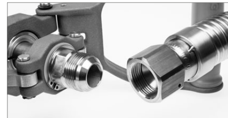
Check if connections correspond in type and size: 1 5/16"-12 SAE J514 37° JIC male / female
