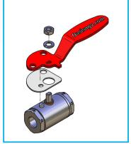
Installation of BV702 Lock Out Handle and Plate
