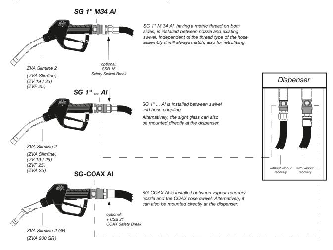
**Note**: Please apply a torque of 25-35 Nm when connecting sight glass to hose assembly/nozzle/dispensers.
