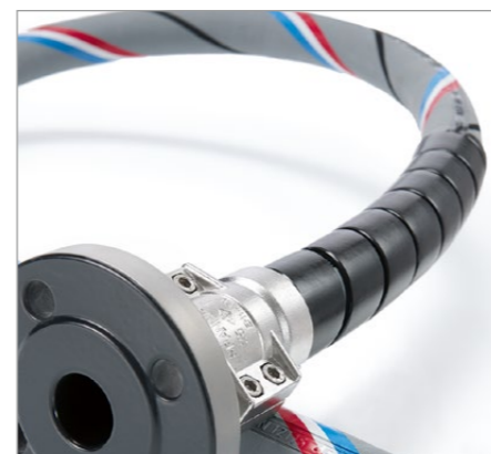
KSS Anti-Kinking Spiral with suitable Spannloc KSS clamps. Patented system for tightly bent hoses - protects the stressed area directly behind the coupling (see Elaflex Information 2.09 E)
